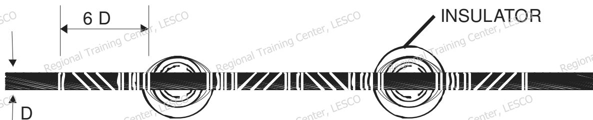
DOUBLE TOP TIE FOR STRAIGHT LINE POSITION
